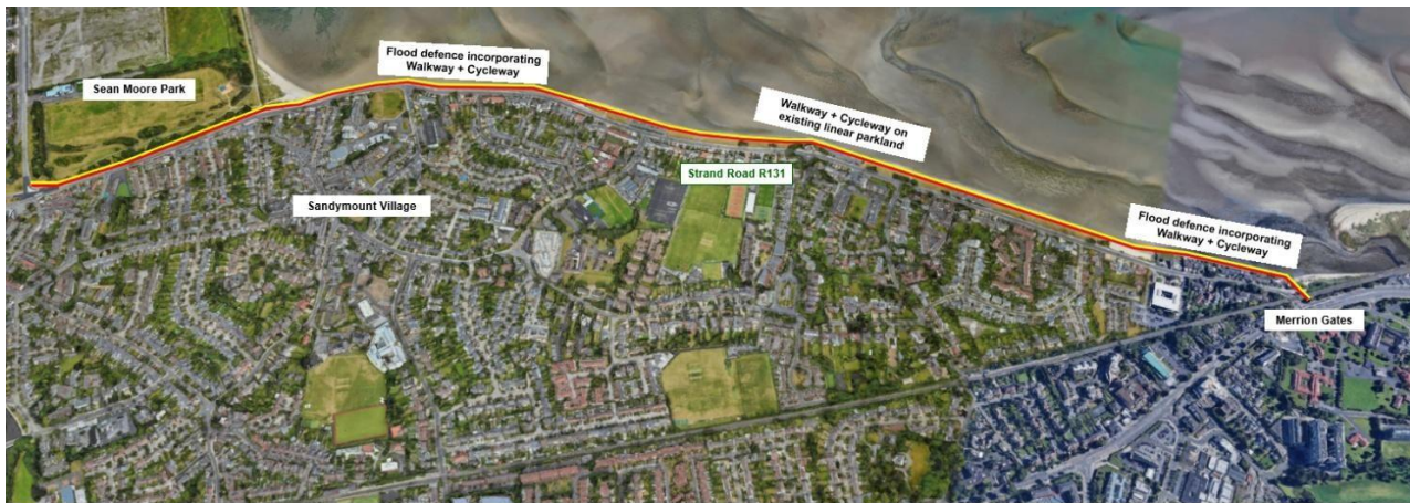
Fig 10: Merrion Gates to Sean Moore Park: a holistic solution that combines flood protection with routes for essential electrical and other infrastructural installations, a continuous traffic free walkway and cycleway together with a permanent way to facilitate ongoing maintenance and repair.
